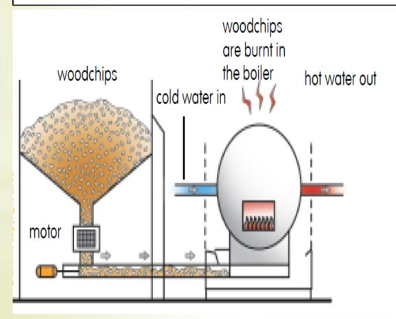
The wood chips are burned in a boiler to heat water, which can be used to heat buildings or make electricity. Household waste, animal and factory waste, and straw can also be used as fuel.
